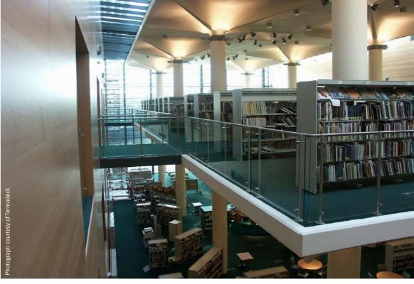
Brighton's Jubilee Library may prove to be one of the most energy efficient buildings in Britain, with the mass of the central concrete structure designed to soak up heat during the day and radiate it back into the surrounding space at night
