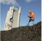
Chipped tyres stockpile to provide for an alternative kiln fuel
