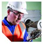
CEMEX UK representative examines Climafuel, an alternative kiln fuel made from household waste
